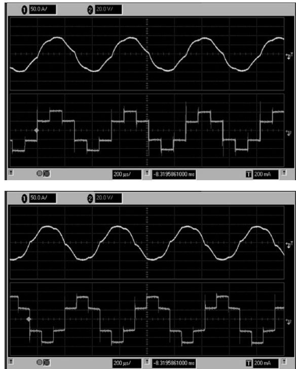
Fig. 21. Oscilloscope traces of phase current (upper traces) and line-to-neutral voltage (lower traces) at 28 kr/min during a 90-A 45-V 6-kW charge (upper photograph) and discharge (lower photograph).
