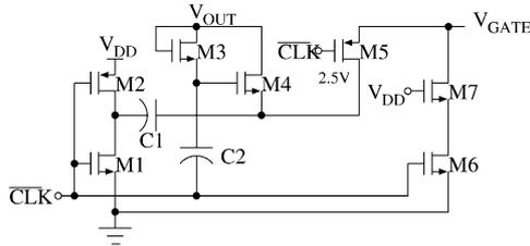
Fig. 7. Capacitor-boost gate drive for the 3:2 converter
