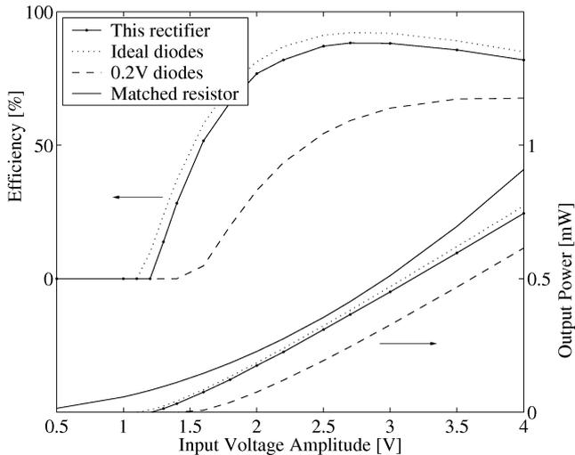
Fig. 16. Power output and efficiency of synchronous rectifier,  $V_B = 1.2V$ ,  $R_S = 2.0k\Omega$
