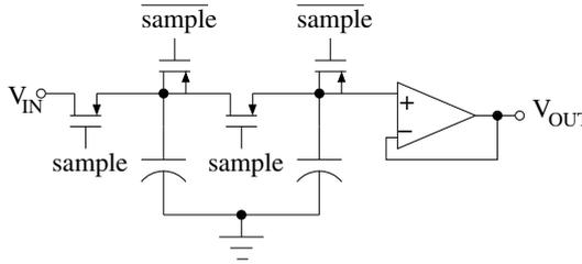
Fig. 13. Low-leakage sample and hold circuit
