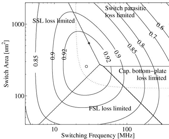
Fig. 5. Optimization contours of the 1:2 converter
